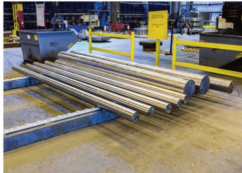
Working with Scot Forge, the OEM was able to keep production moving with an open die forging solution. As the largest procurer of ingots in North America, Scot Forge had the material they needed on-hand, and working with a multistep process, was able to forge a bar, which could then be parted out to produce the forgings the OEM required.
